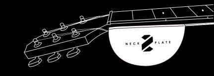
Place the neck plate on a horizontal table, then put the neck in the fixing slot and fix it with a small force
